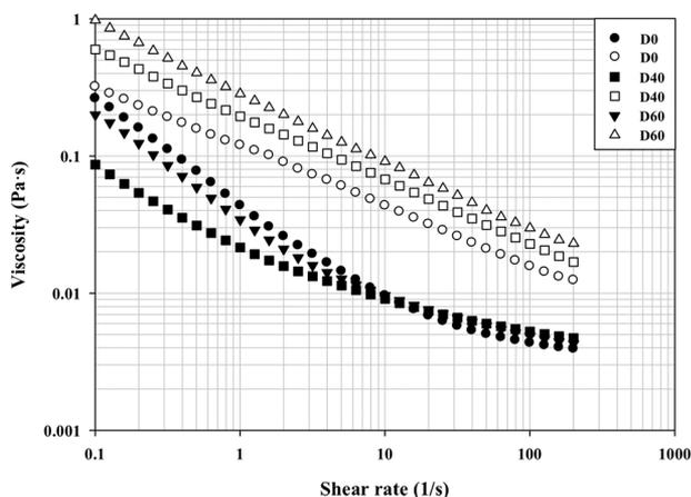
**Figure 5.** Flow curves describing the non-Newtonian shear-thinning flow behavior of fresh (full dots) and reconstituted (empty dots) *A. vera* mucilages treated with different water deficits: D0=aloe without water deficit; D40=aloe with 40% water deficit; and D60=aloe with 60% water deficit. Modified from Minjares-Fuentes et al. (13).
