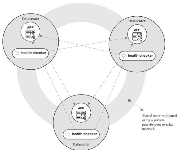
Figure 3: Illustration of Akash’s overlay network
