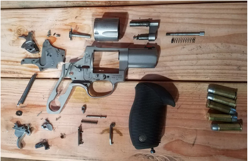
Overview over the Taurus Tracker torn down to the frame.
