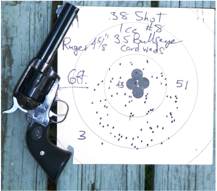
Shotshell pattern from a 4-5/8" Ruger Vaquero. Photos by C.E. Harris.
