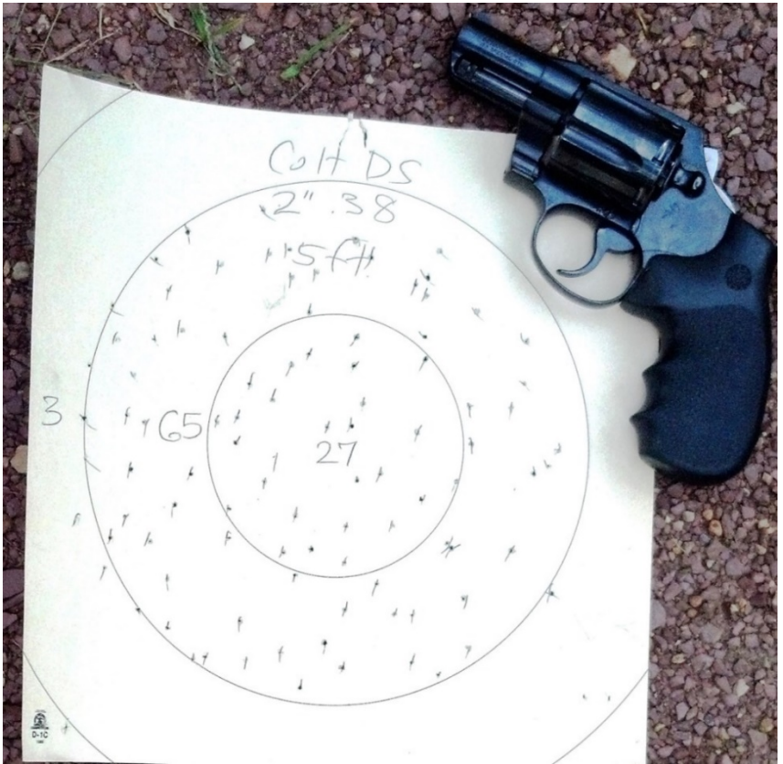
Shotshell pattern from a 2" Colt Detective Special.
