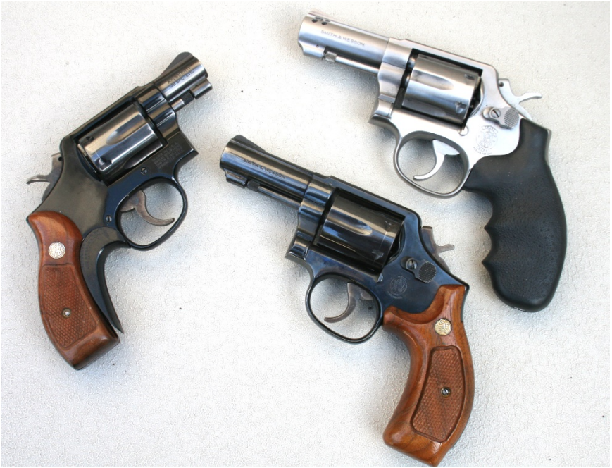
The trio of revolvers clockwise from left to right: S&W M12 Airweight 2", S&W M64 3" and S&W M547 3".
