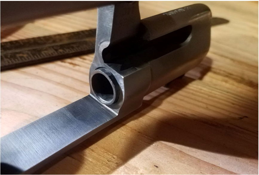
View of the minor flame cutting and forcing cone on the Tracker.
