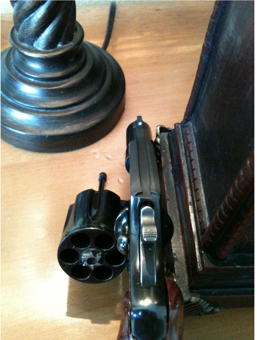
Seamless dovetail front sight and nice charging hole chamfers.
