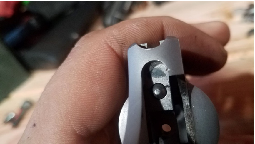
View of the peen holding the firing pin in on the tracker.
