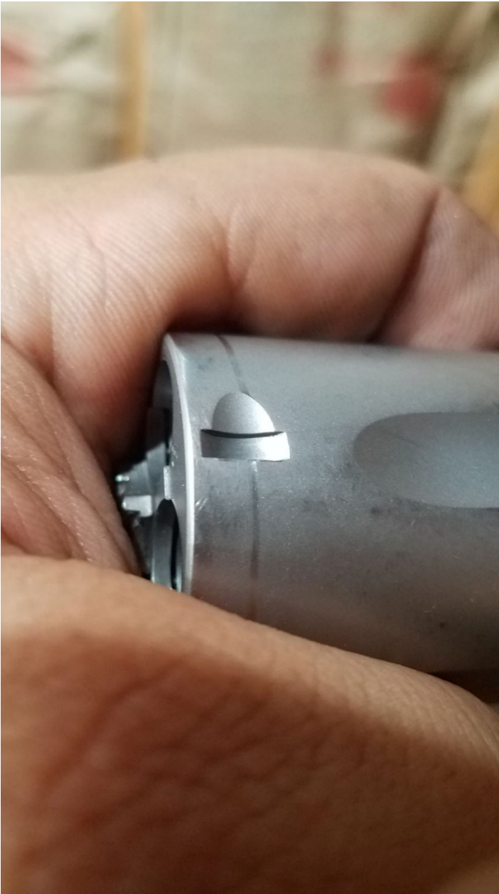
View of the burrs on the cylinder latch notches.
