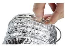
Then place the hose over the extractor port on the back of the spray booth and release the spring clip to hold the hose in place.
